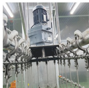
Processing line driving unit
