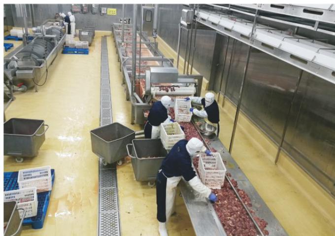
Heart & Gizzards processing belt chiller, lifting conveyor
