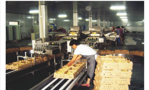
Counting and packing unit with two-paths
